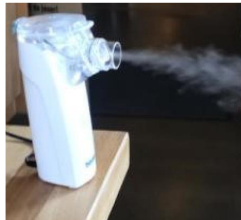
Fig. 23 Nebulizer is used to form a spray of salt solution droplets, drying fast, forming a cloud of 30 nm particles, about 80'000 per cc
