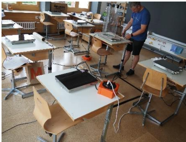
Fig. 22 Researcher installs the particle source at one desk, all other desks have particle counters and heated plates to simulate the students
