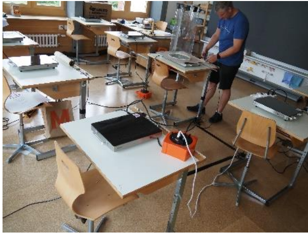
Fig. 22 Researcher installs the particle source at one desk, all other desks have particle counters and heated plates to simulate the students
