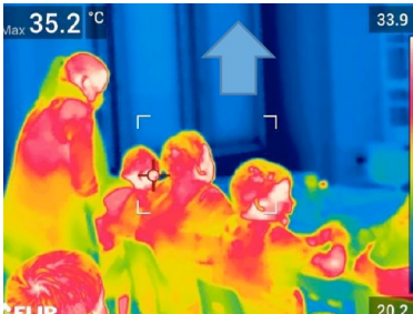
Thermal drift by body heat 50-100 W, 2-5 cm/s
