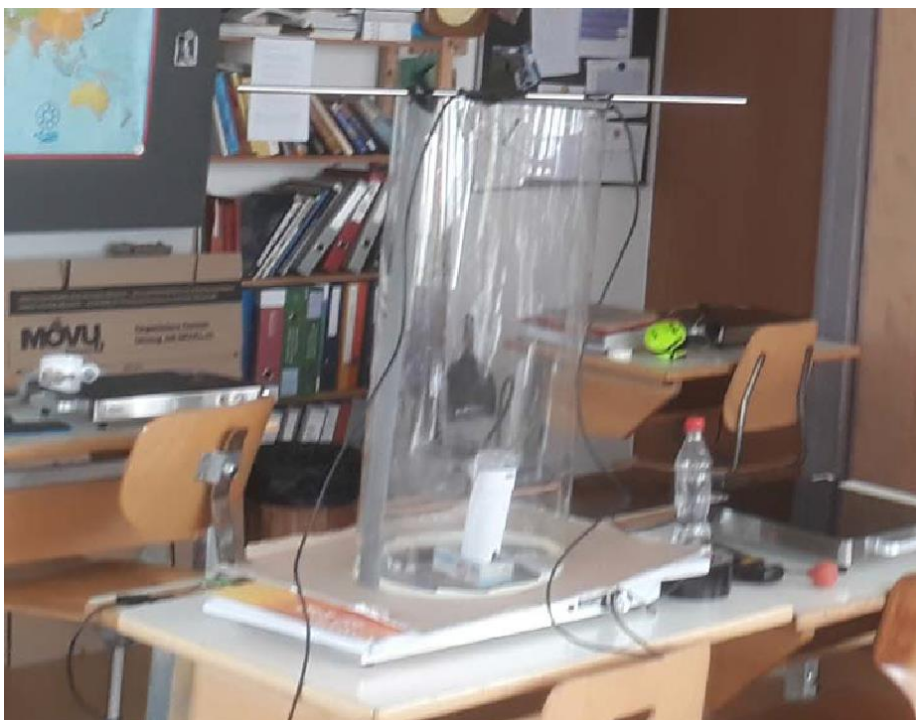
The nebulizer is used to spray saline particles. This simulates the mode of action and the spread of aerosols in the room
